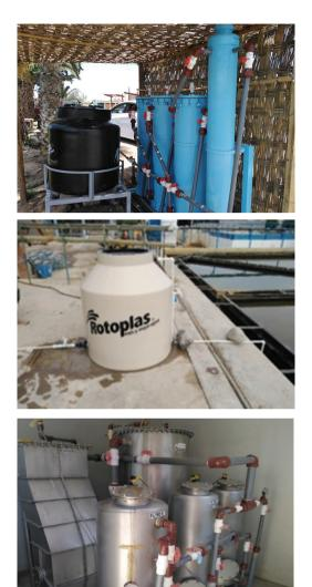
The granular material was incorporated in multimedia filters, avoiding pre-treatment by means of a direct water intake bypass from collection into the filtration units. Given the high turbidity values of the outflowing water (the regulations recommend less than five Nephelometric Turbidity Units), it is necessary to improve the treatment with a refining unit at the end of the process.
